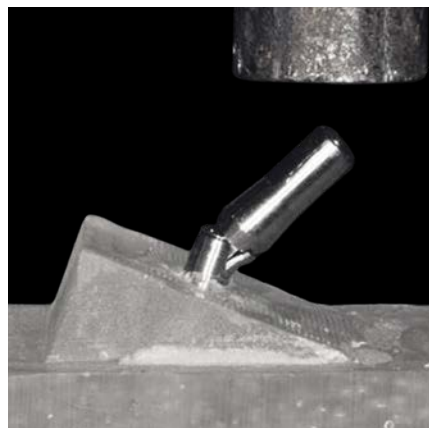
2. Abutment-implant connection during the mechanical failure
